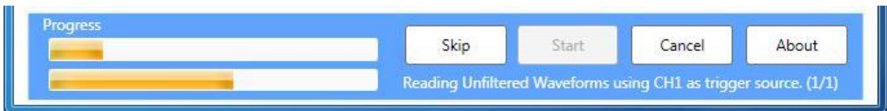
Figure 44 Progress bar latched orange after losing phase reference source
