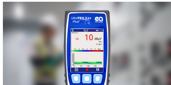
Figure 1: Screenshot of UTP2 display showing a positive indication of ultrasonic discharge activity.
