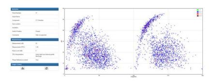
Example of internal void PD measured using the TEV sensor. Asset information can be transferred and sent to EA Technology or your in-house PD experts for review.
