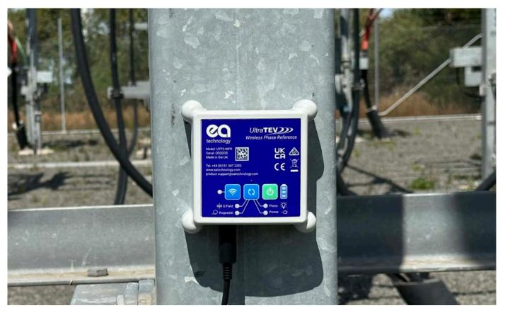
Wireless Phase Reference being used in situation.
