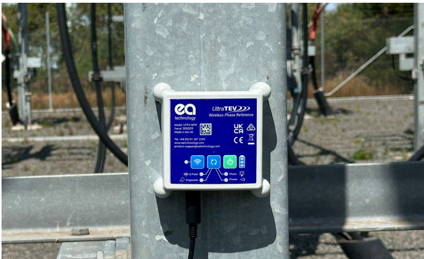
Wireless Phase Reference being used in situation.
